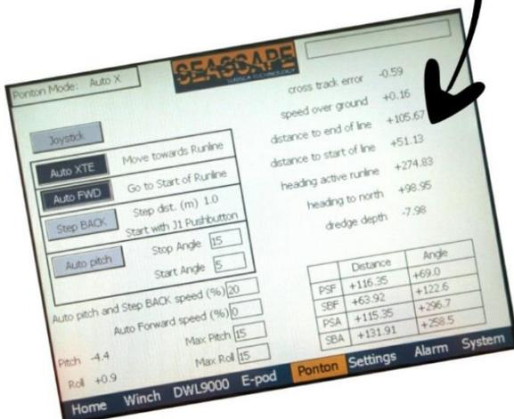
**Seascope developed an PLC software positioning system to position a vessel or pontoon with a 4 point mooring system.**
