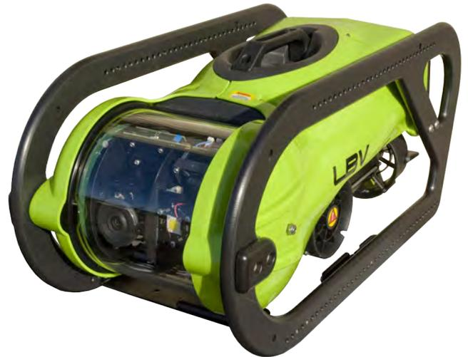
With powerful brushless thrusters, small diameter low drag tether, and a very stable and maneuverable platform, the SeaBotix LBV200-4 Series is the most capable and featured system in its class. The LBV200-4 is an extremely portable system with a host of options offering a turnkey solution for a demanding range of applications.
